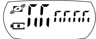
test pattern 2 (alternate segments activated)
